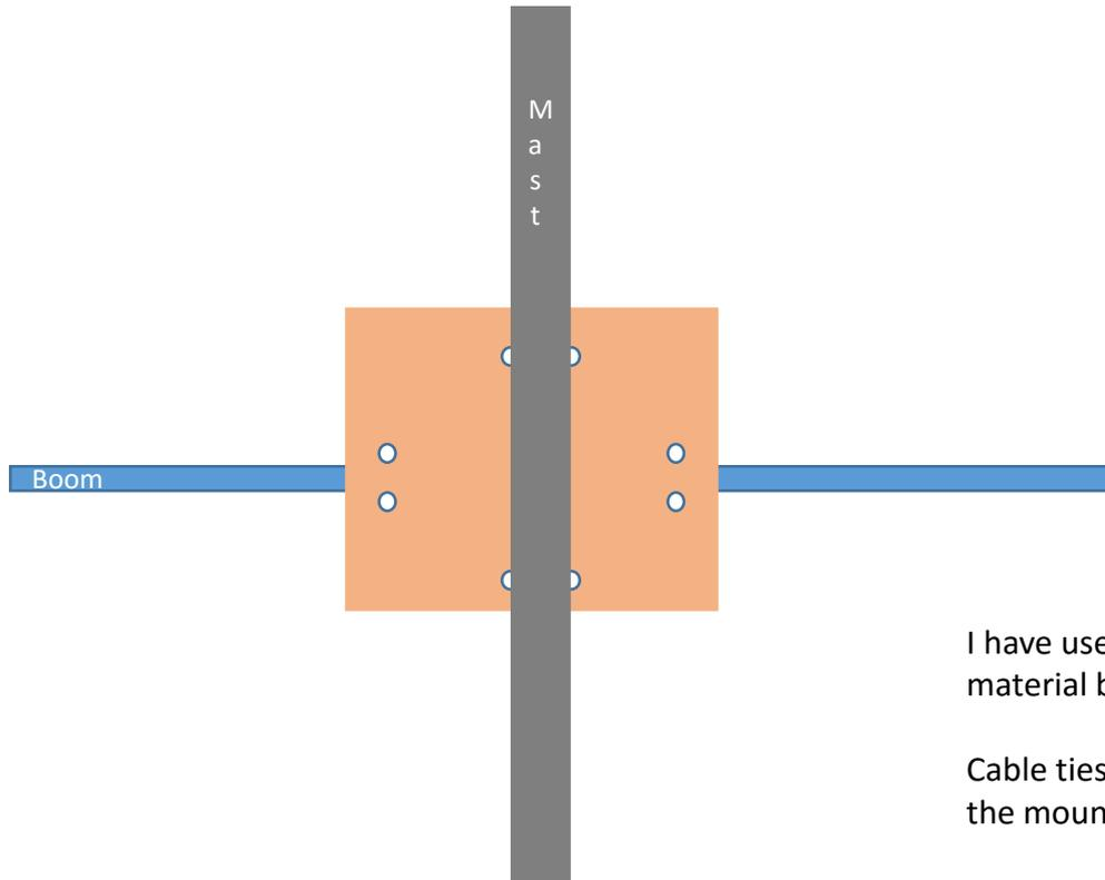
I have used 5mm thick Pertinax plate as bracket material but any stiff enough material is ok.
